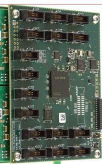
Fig. 2 The Star-Hub module enables systems with up to 128 channels.
