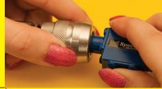
3. Push "Lock Nut" forward and engage the Push-On end of the Adapter with the mating female. Back nut must be released.
