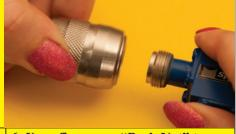
6. Keep fingers on "Back Nut" to ensure that "Lock Nut" cannot slide rbackduational the assmission off.
