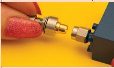
4. To disconnect, just pull the connector off.
